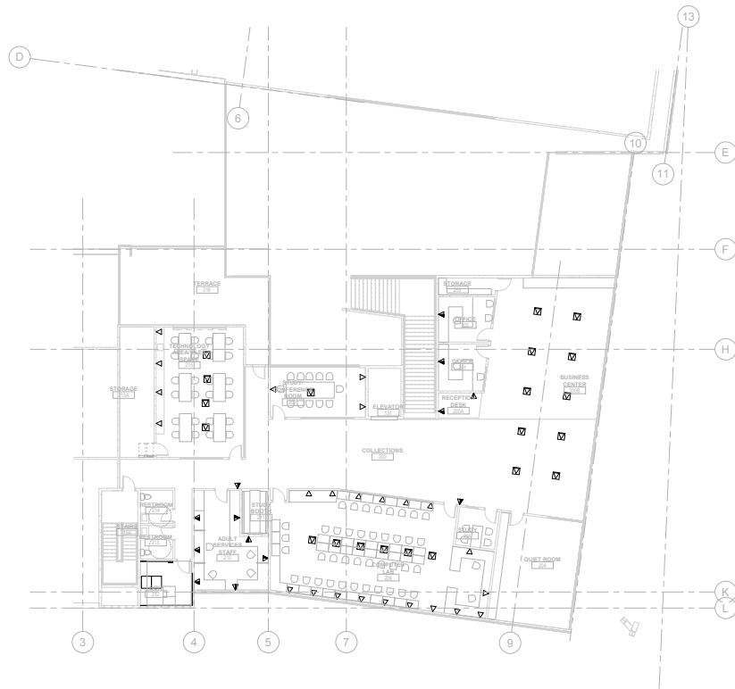
1 COMMUNICATION NETWORK PLAN - SECOND FLOOR - AREA B SCALE: 3/32" = 1'-0"
